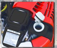
Extended Oil Drain Plug. Easy to change Oil. Fill 80ml oil up to the bottom of Oil Inlet(Stop adding oil when you see the oil at the bottom of the oil Inlet.)Do not fill oil up to the mouth of the Oil Inlet.
